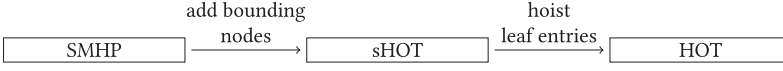
Fig. 6. Relationship between SMHP, sHOT, and HOT and how to transform partitionings created by SMHP into HOT structures.
